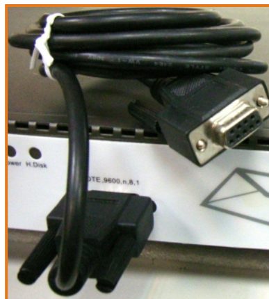
Figure 7 Connecting the Cable to the Port and Placing It on the Device
